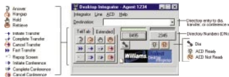
Desktop Integrator's User Interface takes up only a small corner of the desktop and lets agents make, answer, disconnect, transfer, and conference calls — without ever touching their phones.
